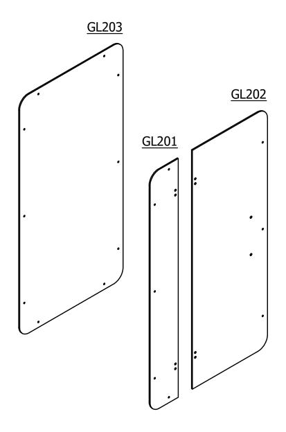
GL201 - Sidelight glass panel has 5 holes for assembly by M10 countersunk screw FS203 with plastic socket cap FS204 two pairs of holes for door hinges assembly
