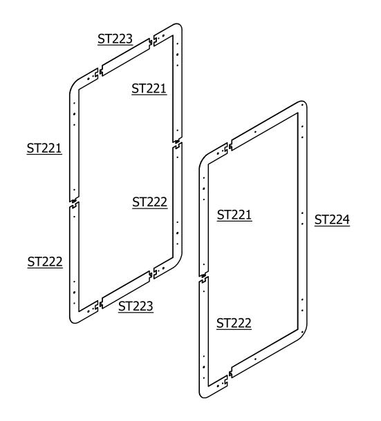
ST221 - Frame metal part (1 on front, 2 on back) with self taping screws (FS201 x 8) per piece.
